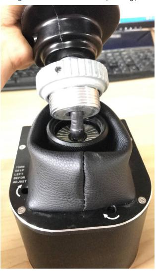
16. Do not twise your grip, just turn and tighten the screw below! Tighten the whole grip onto base.
