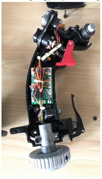
5. Untie the wire, unplug the wire and unscrew the screw as arrow pointed.
