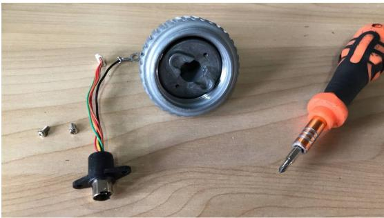
7. Replace the connector wire, make sure you left 4cm (2 inches) out at the bottom
