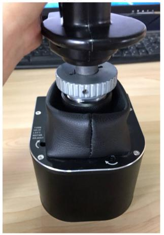
17. Make sure the screws are align on the base screw, use 2.5MM Allen screwdriver tighten up the whole set. You are good to go.
