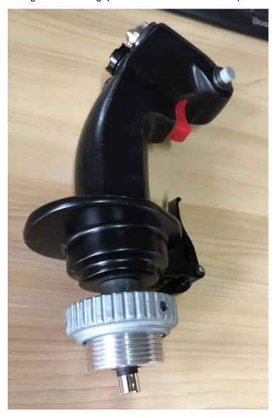
15. Aligned the connector to the base, avoiding pull it out too much from the base.
